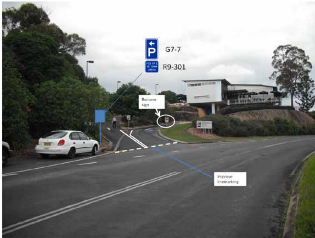
Figure 4 - suggested signage and linemarking changes
