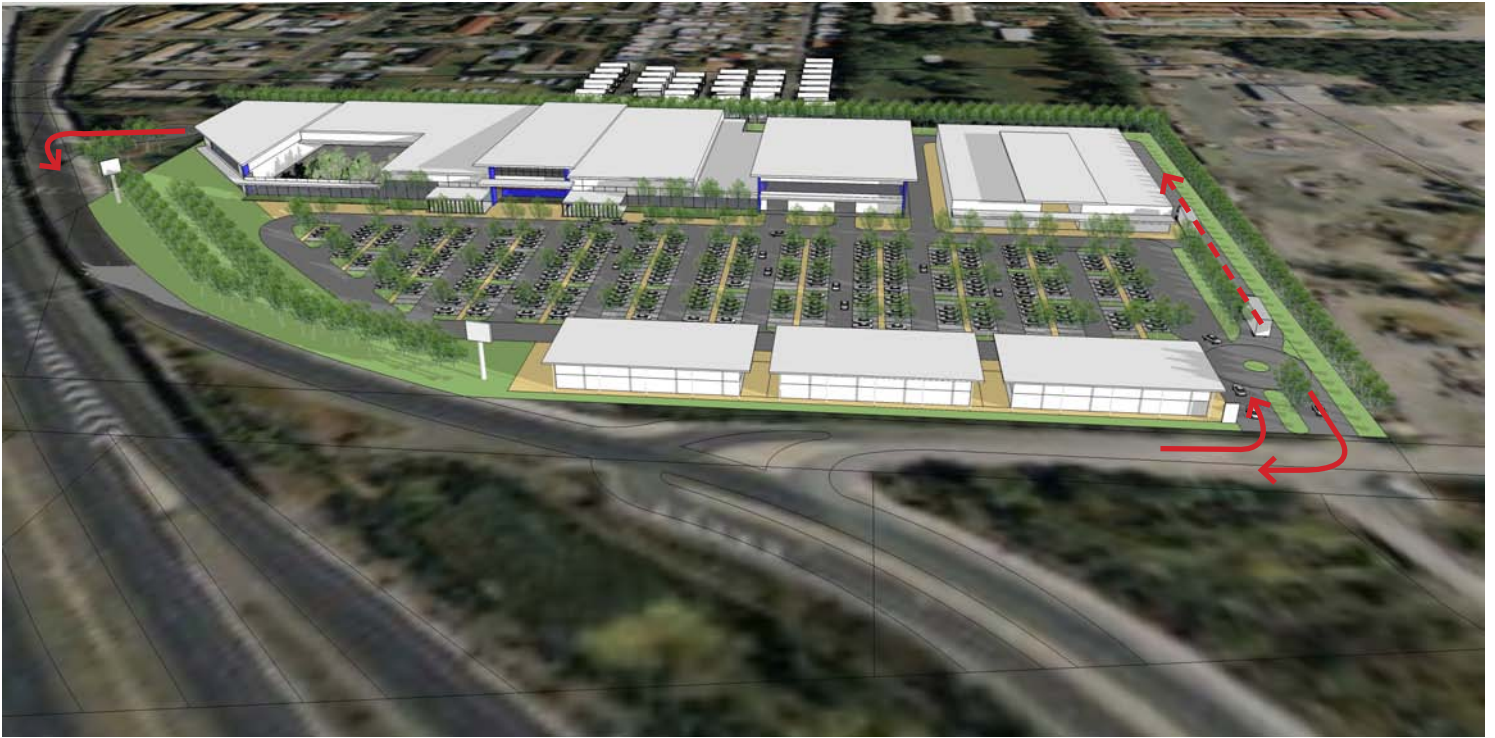
Figure 8.3 - Site configuration - The subject site has a number of constraints including building height (13.6m), singular point of access (off Parkes Drive), flooding (northern portion) and proximity to the waste water treatment which influences where building envelopes can be positioned. There is opportunity for a larger floor plate development adjoining the southern boundary, a multi-unit development in the south west corner of the site and a narrow floor plate development along the sites northern boundary around a centralised car park area. Perimeter service vehicle lane would separate service and customer vehicle movements. Landscape buffers to adjoining boundaries will be required and there is opportunity to continue a strong landscaping frontage to Rose Street.
