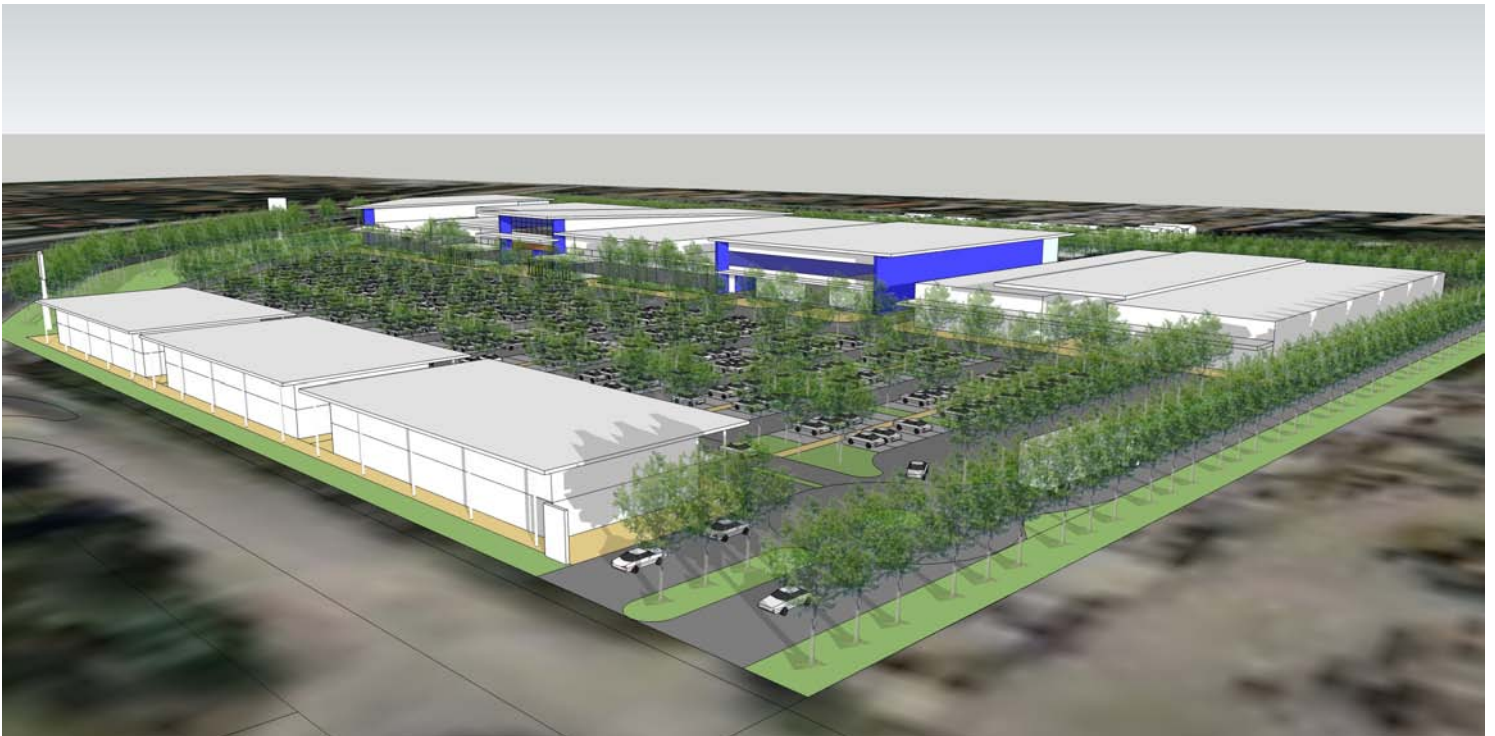
Figure 8.4 - Centralised car parking area and water sensitive urban design- A centralised landscaped car park area which adopts water sensitive urban design principles could serve all business park land uses. Given the amount of hardstand area that would be generated from required car parking numbers, this needs to be offset by a strong landscape plan with street trees and public domain and residue landscape area which would allow for some stormwater infiltration.
