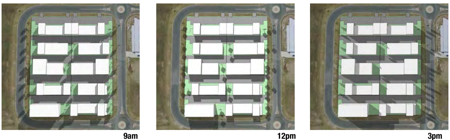
Figure 5.4 - Shadow Diagrams - Modelling of shadow diagrams enables a review of solar aspect during different times of the day making it an important design tool for siting and configuring building layouts. It also enables a review of the potential for overshadowing neighbouring allotments and buildings.
