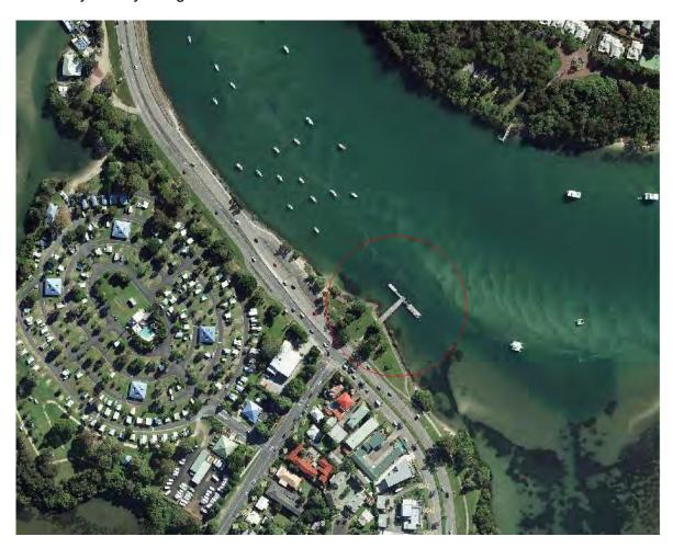
The jetty consists of a timber wharf with two floating pontoons attached. One pontoon provides facilities for vessel sewage pump out. The facility is used frequently by owners of vessels moored nearby for loading and unloading passengers and equipment/supplies.
