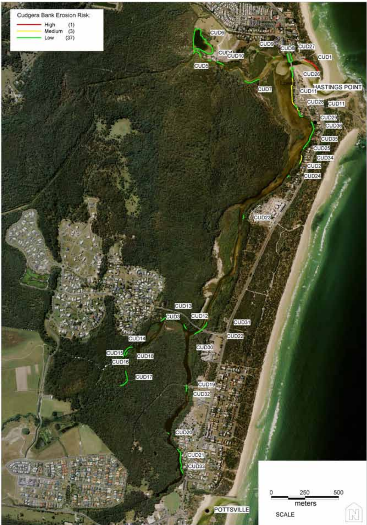
Figure 14: Cudgera Creek Bank Erosion Risk (refer Appendix 3 for further details)
