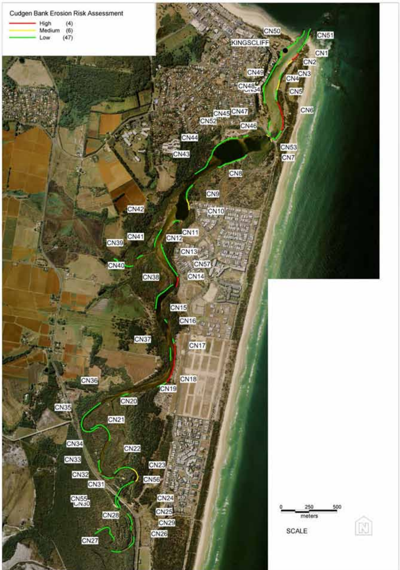
Figure 13: Cudgen Creek Bank Erosion Risk (refer Appendix 3 for further details)
