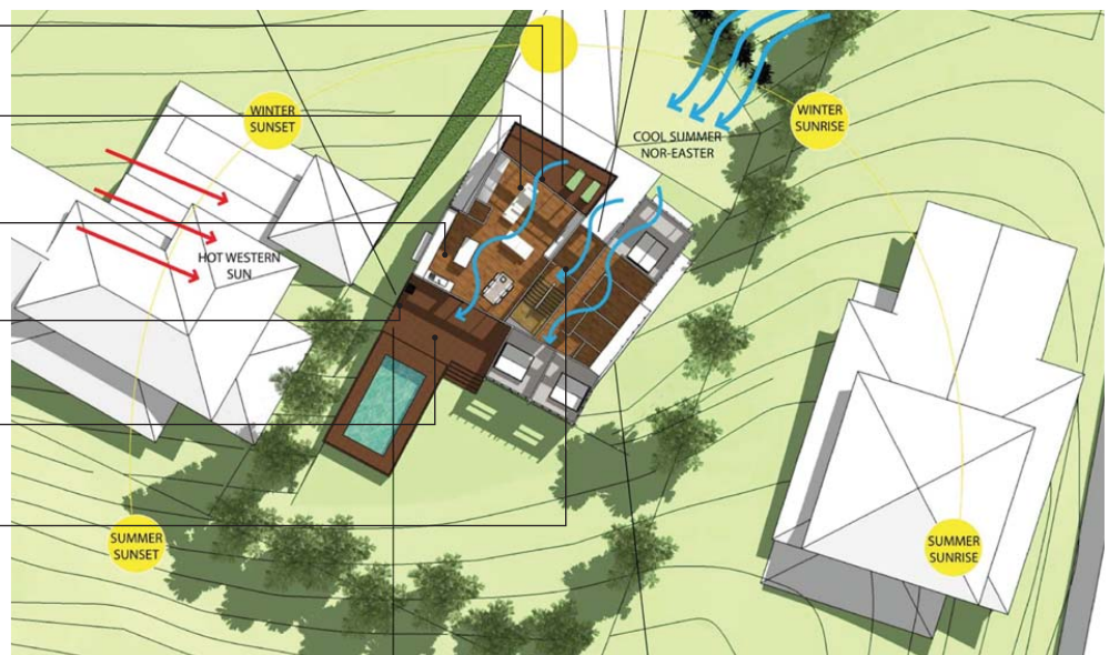
Sample Passive Design - Illustrate and notate the principles of passive design as part of a site analysis.
