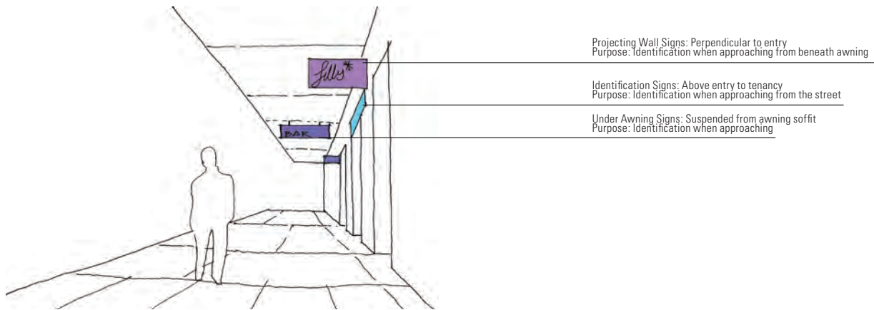
Figure 4-13: Under awning signage
