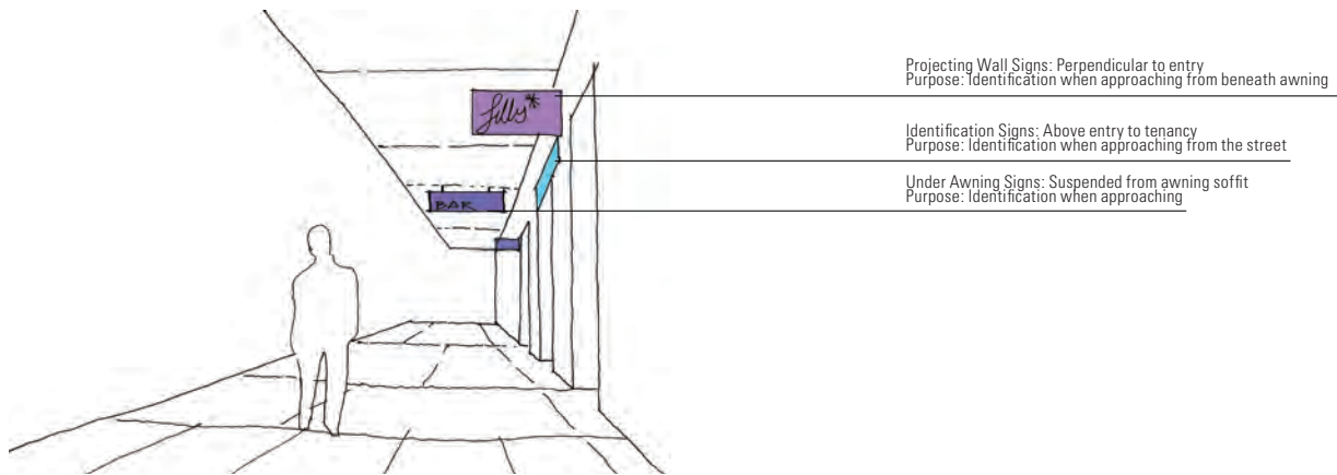
Figure 4-13: Under awning signage
