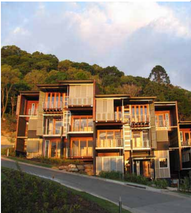
The massing of buildings needs to be broken down to step with the topography.
