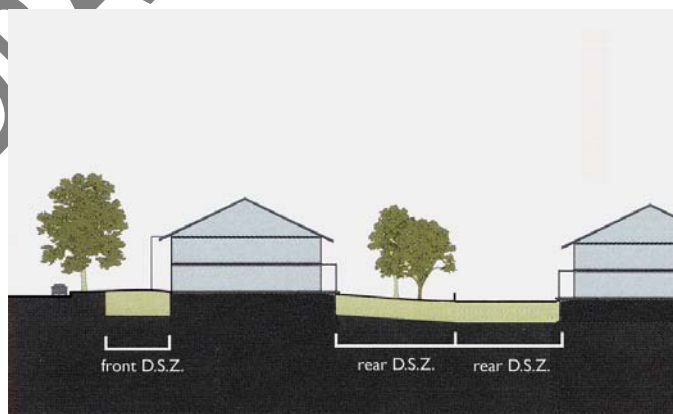
Deep soils zones fit neatly around the building without obstruction either above or below by built elements such as carpark ramps, impervious surfaces or terraces
