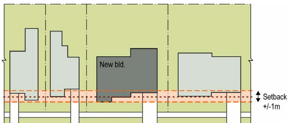
Setbacks are designed to provide a consistent alignment along the street.
