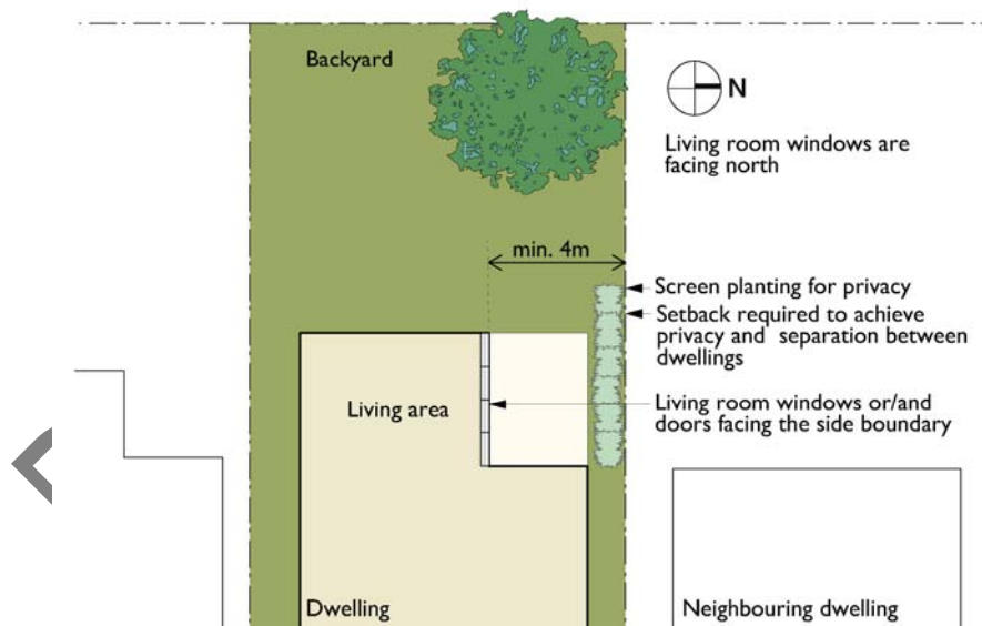
On lots with north to the side boundary living room windows can face the side boundary if set back.
