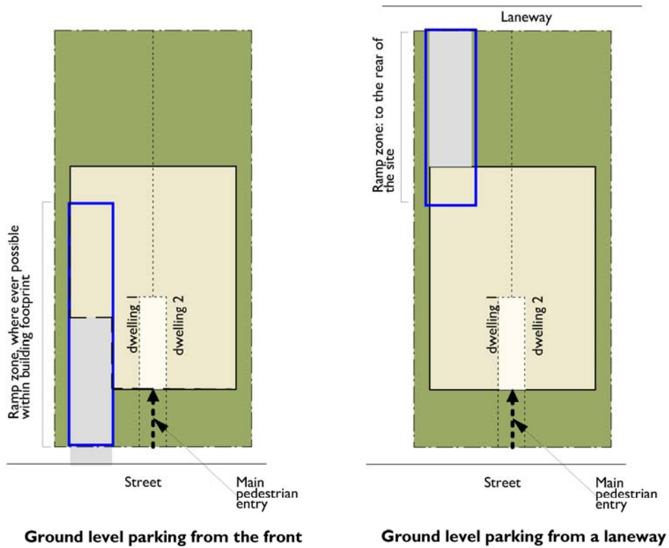
Indicative layouts for a Small Residential Flat Building with two dwellings per floor.
