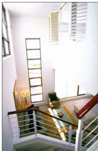
Double height ceiling spaces can significantly increase light penetration into narrow or one-sided apartments as well as add to the quality of the internal space.
