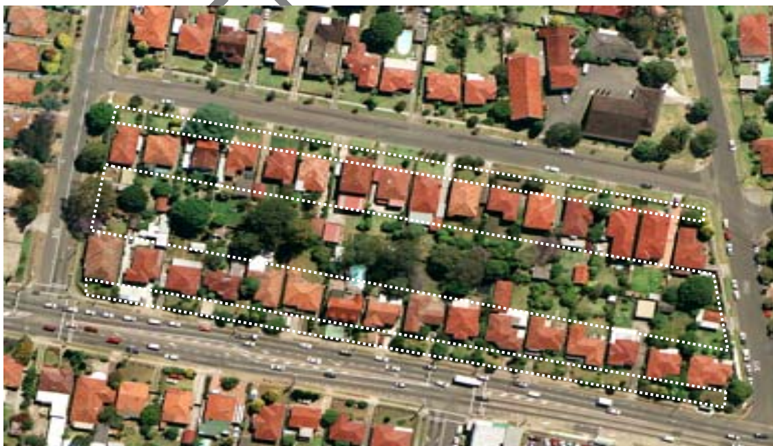
Existing mature trees are generally located to the rear of lots by locating the Deep Soil Zone here it is possible to retain mature trees.
