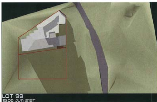
99 TWEED COAST ROAD BOGANGAR : PROPOSED MULTI-DWELLING REDEVELOPMENT SHADOW DIAGRAMS FOR JUNE 21 PREPARED BY NEOCONCEPTS FOR GINA GHIONI ARCHITECT 22 NOVEMBER 2007
