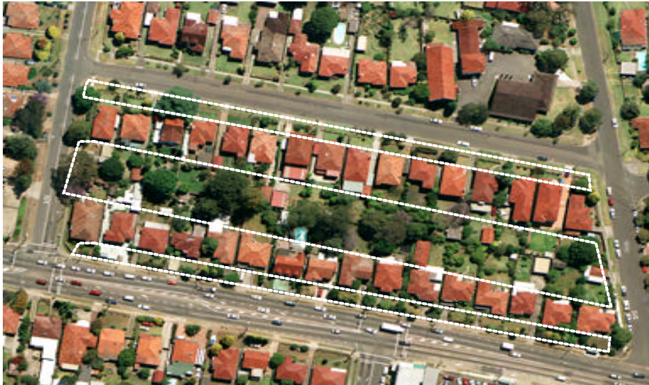
Existing mature trees are generally located to the rear of lots, by locating the Deep Soil Zone here it is possible to retain mature trees.
