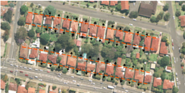
In established residential areas all buildings are oriented to the front and rear of lots so that privacy and outlook are coordinated across the block, the street and between neighbouring buildings.
