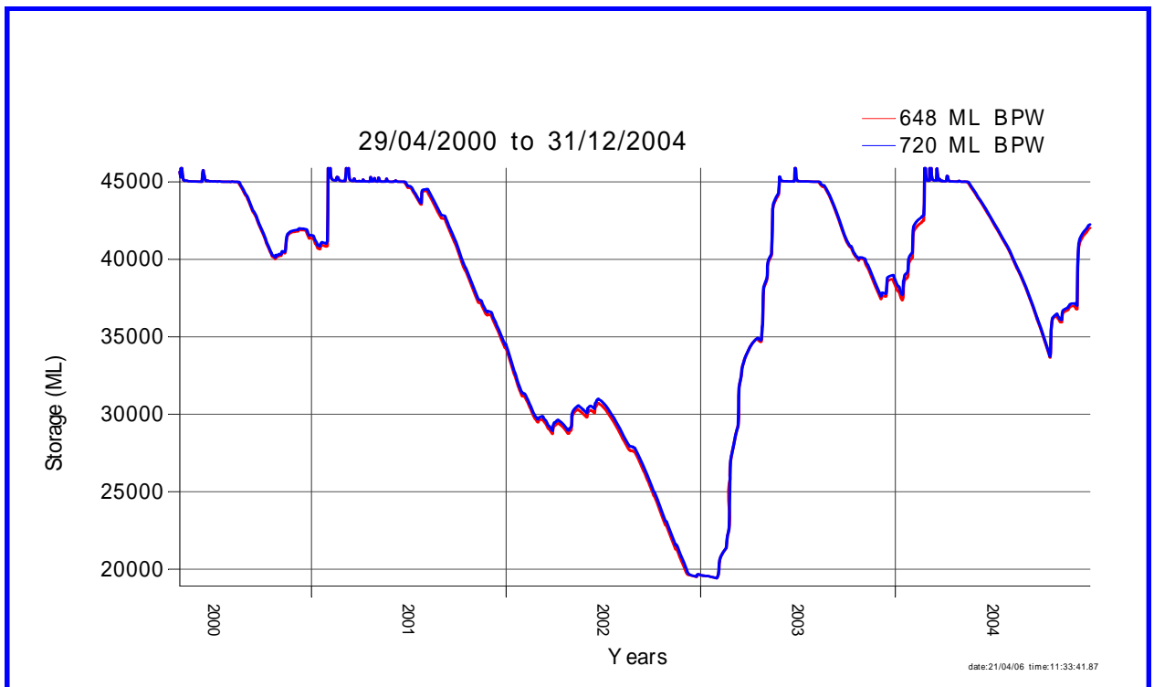
Figure 8.4: Clarrie Hall Dam Storage for 648 and 720 ML of Bray Park Weir Capacities
