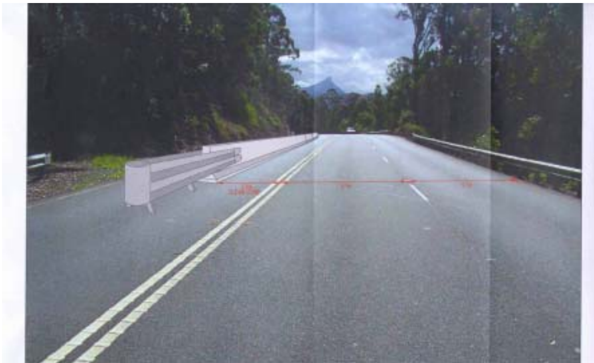
Photograph 4. Indicative view of roadway past cutting with recommended barrier
