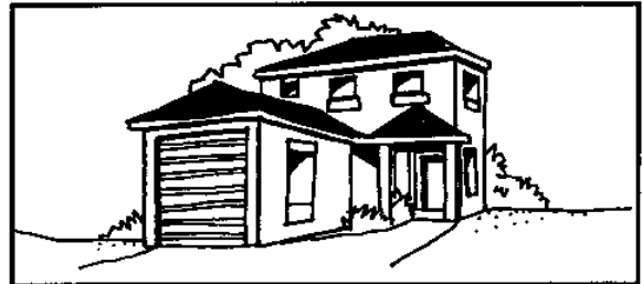
Poor relationship to street - the garage dominates the dwelling when viewed from the street.
