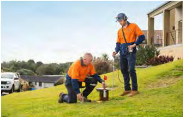
Technicians using special acoustic technology were on the hunt to detect water leaks.
